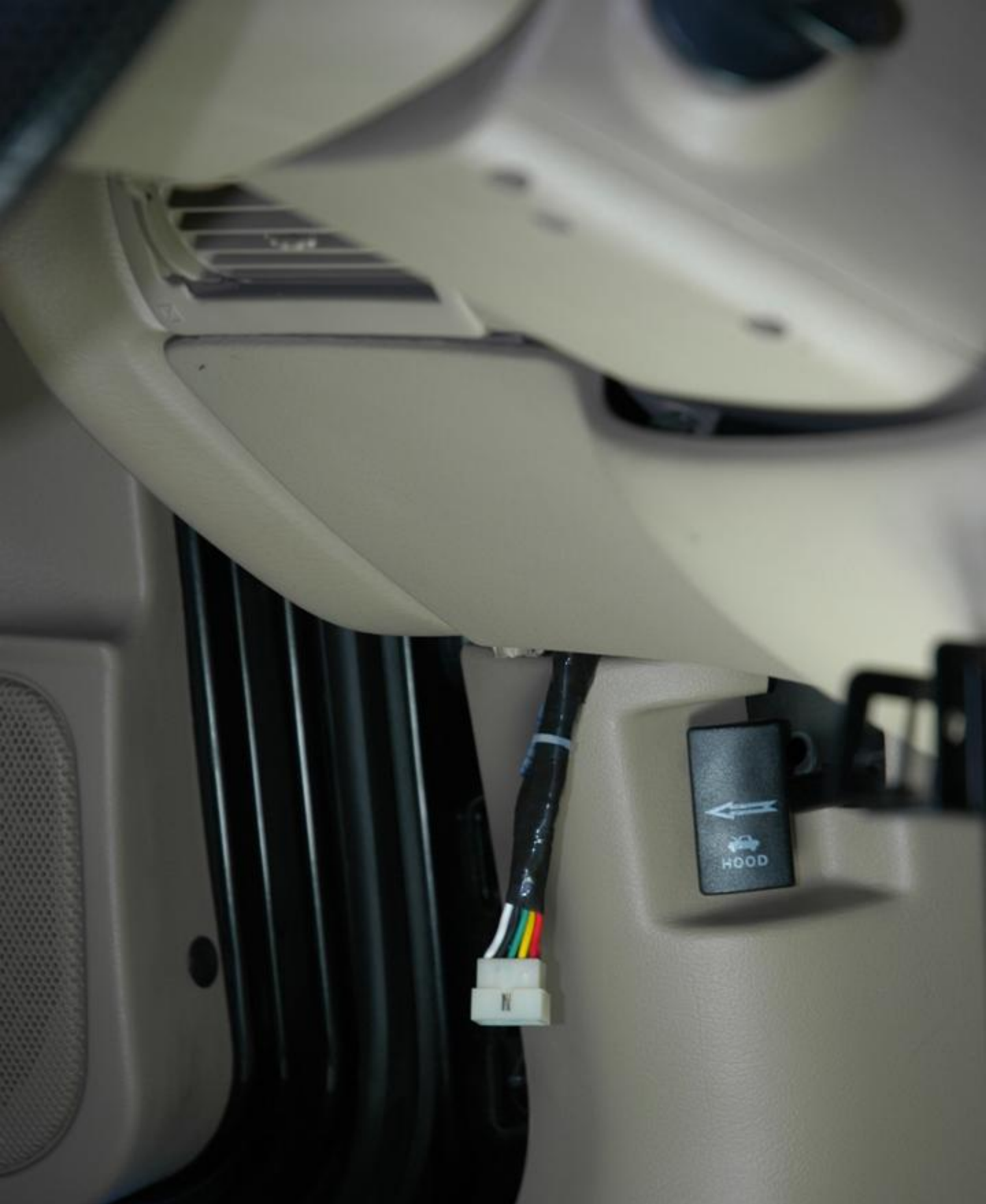
A-pillar harness terminated with Molex 15-pin connector
