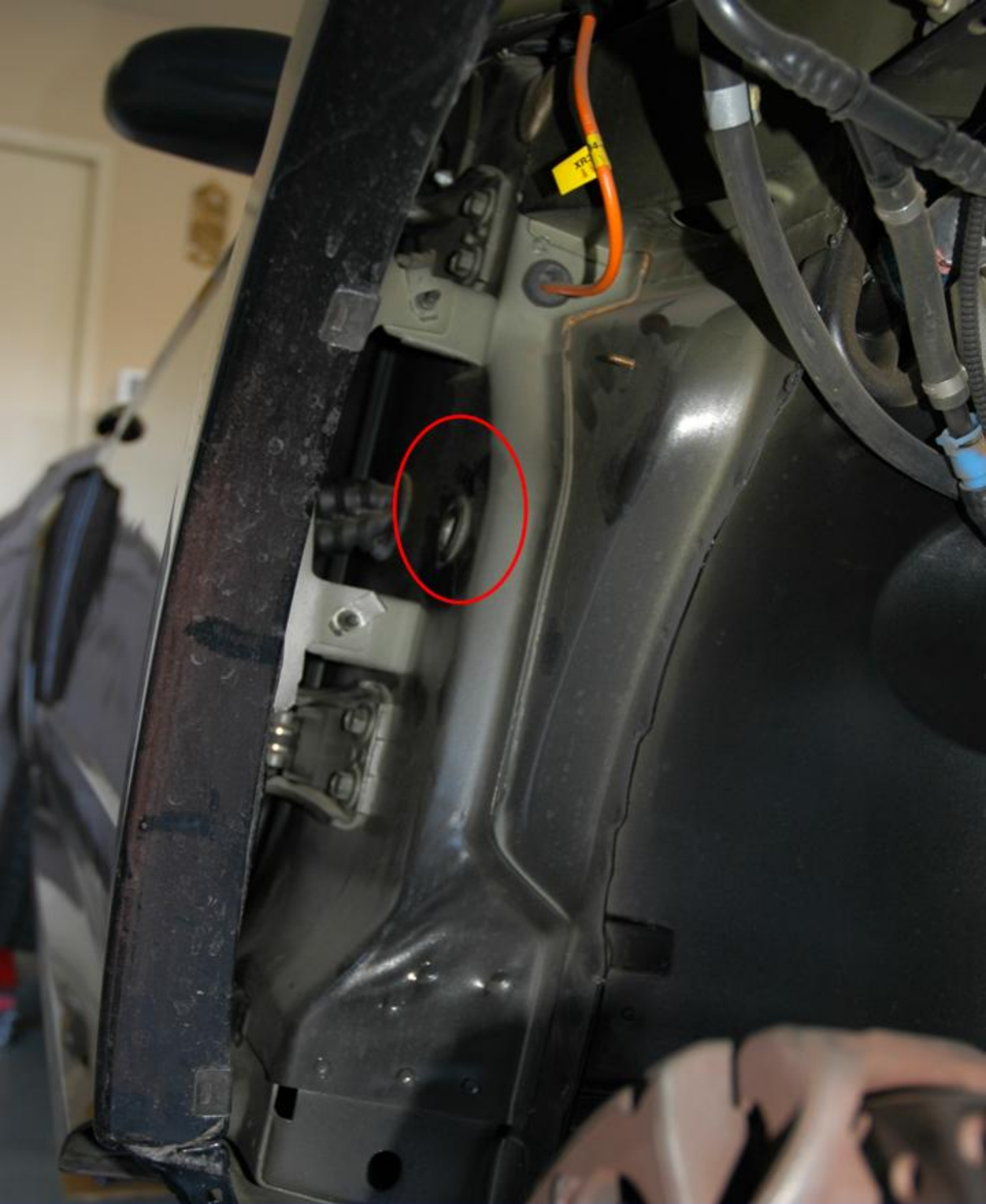
Existing passenger side grommet used for wire feeds
