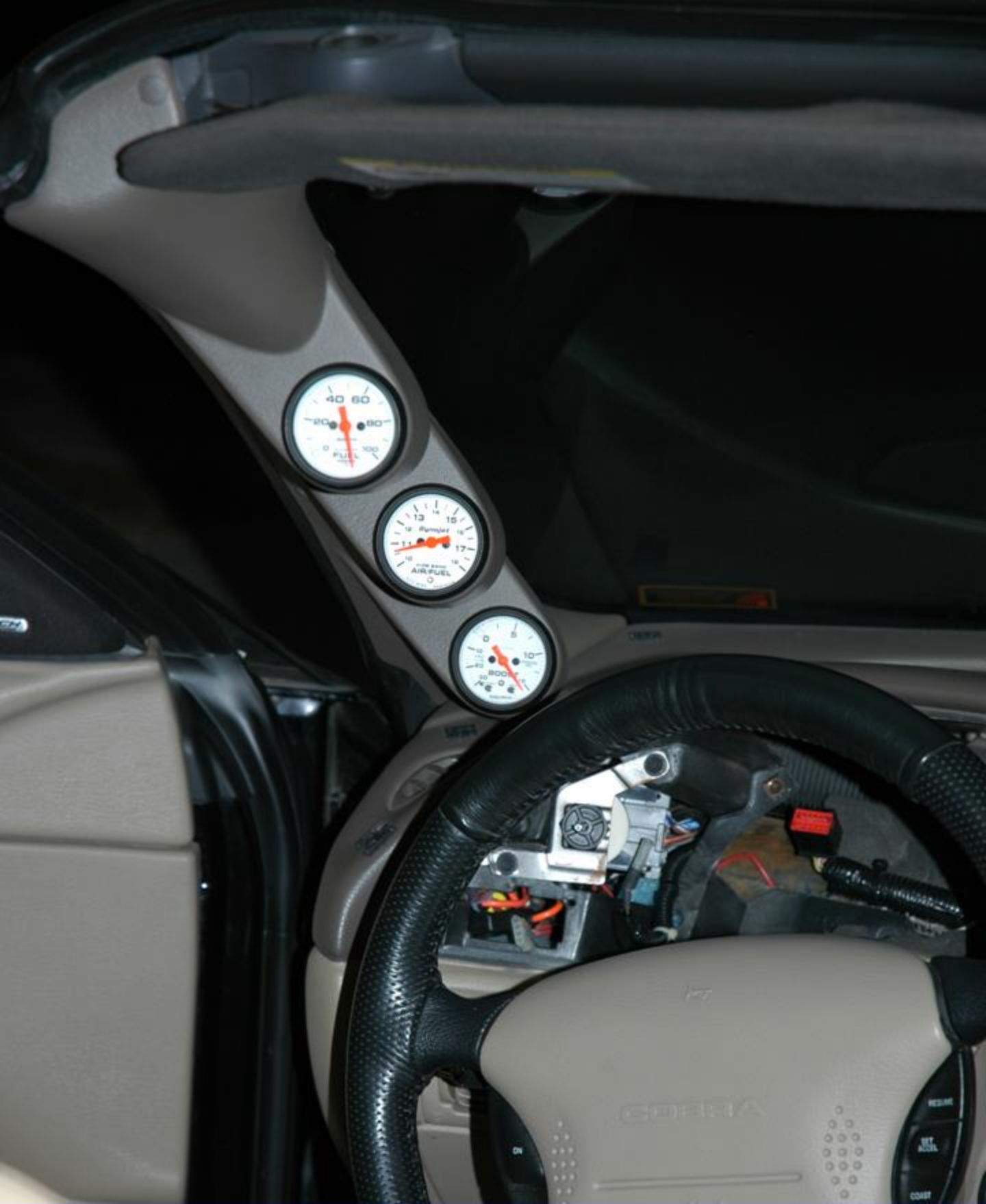
Gauges installed in A-pillar
