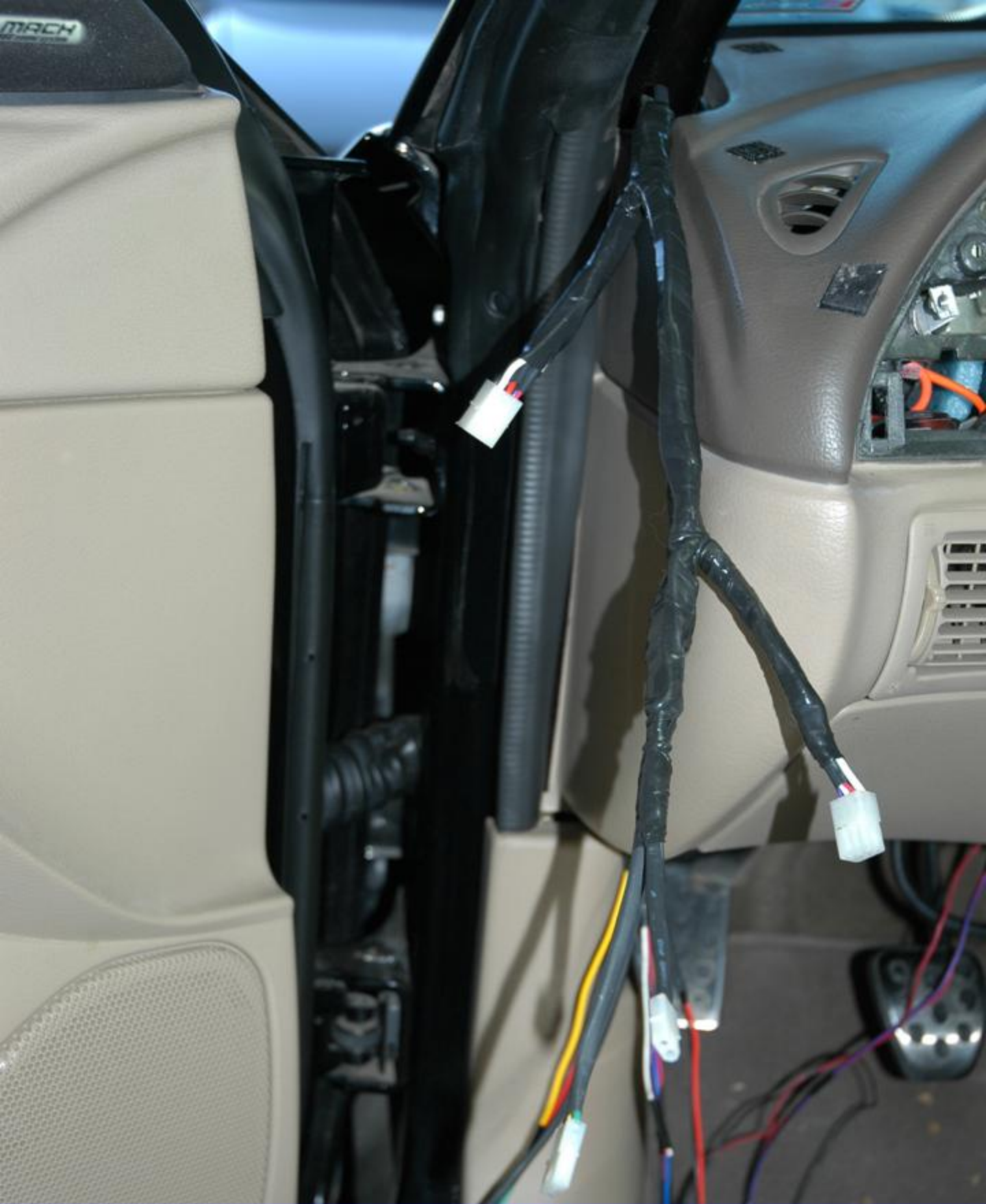
Lighting circuits added and individual harnesses bundled together
