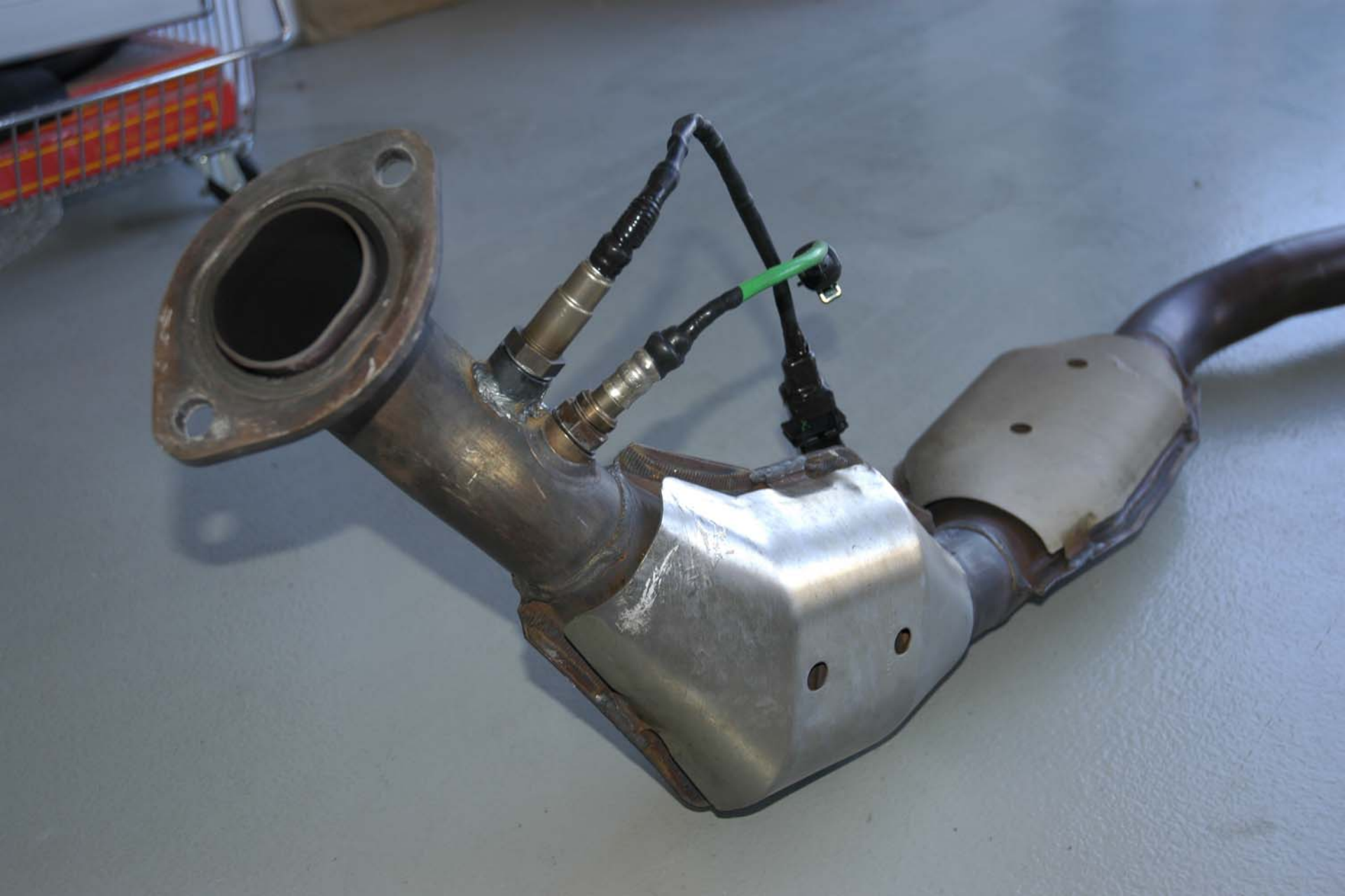
New wideband O2 sensor installed on right down-tube of mid-pipe
