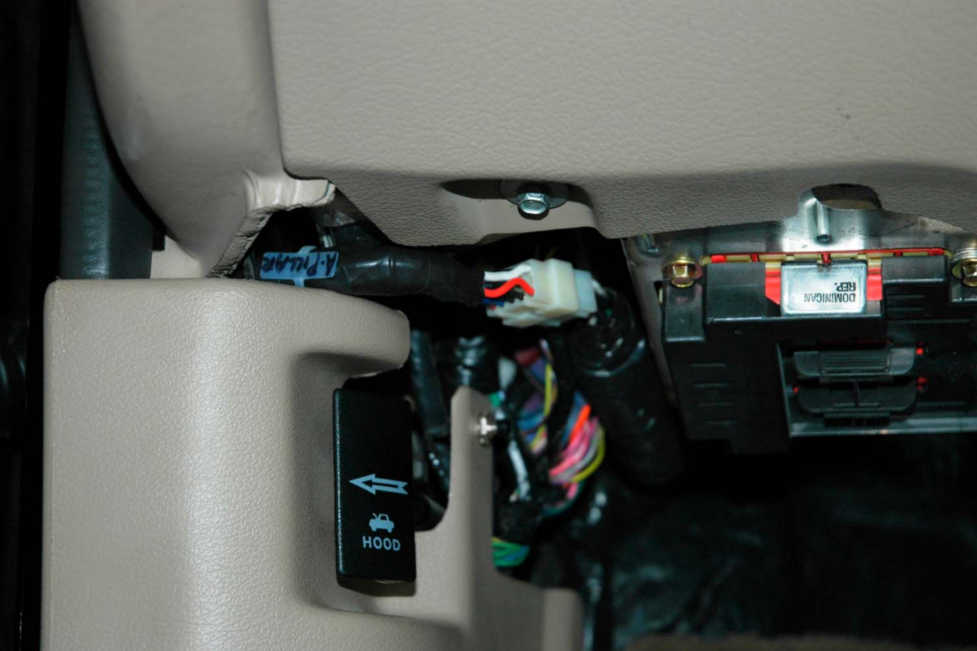
A-pillar harness connected to sending units & vehicle electrical system
