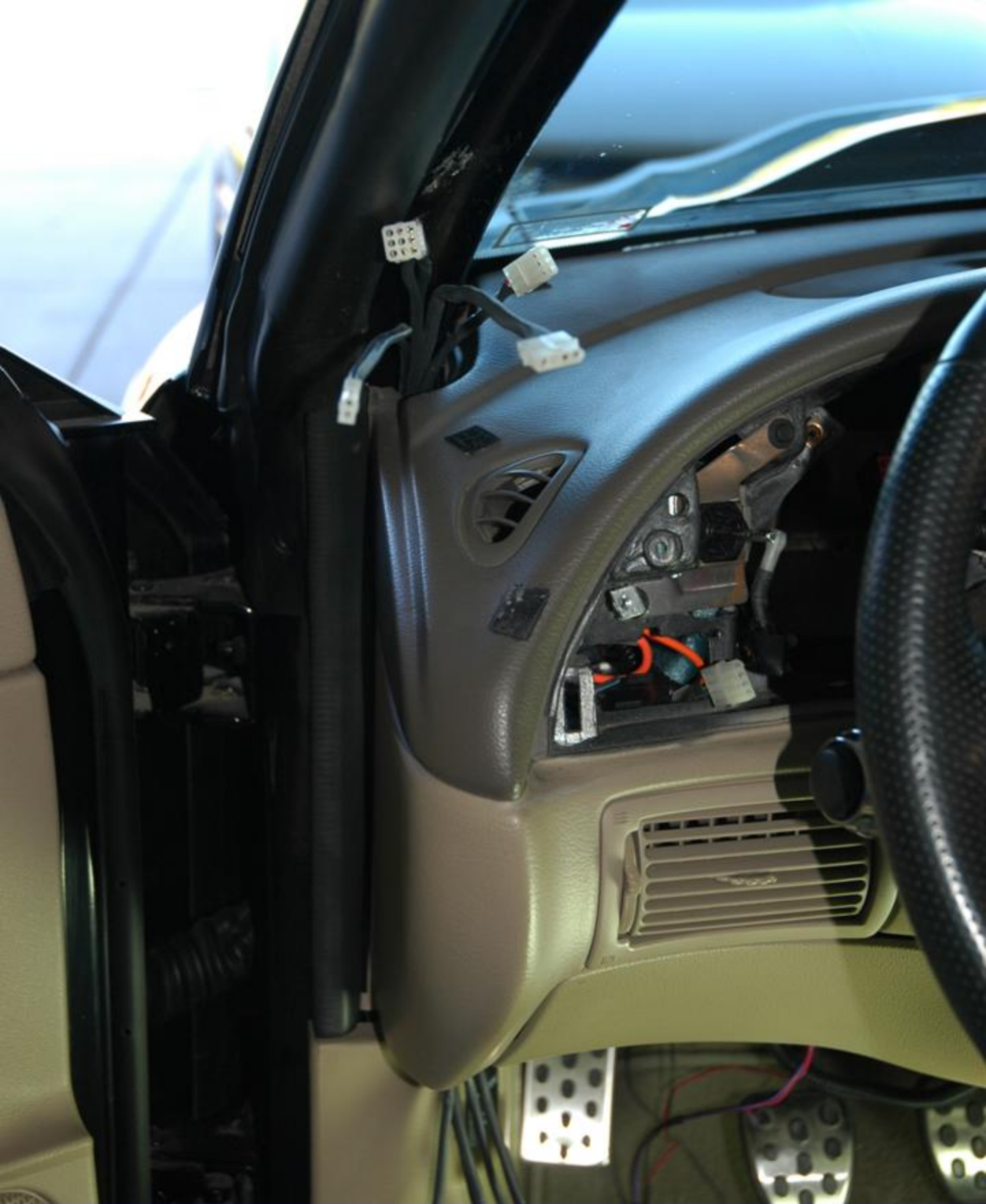
Gauge harness pulled down through opening at A-pillar base
