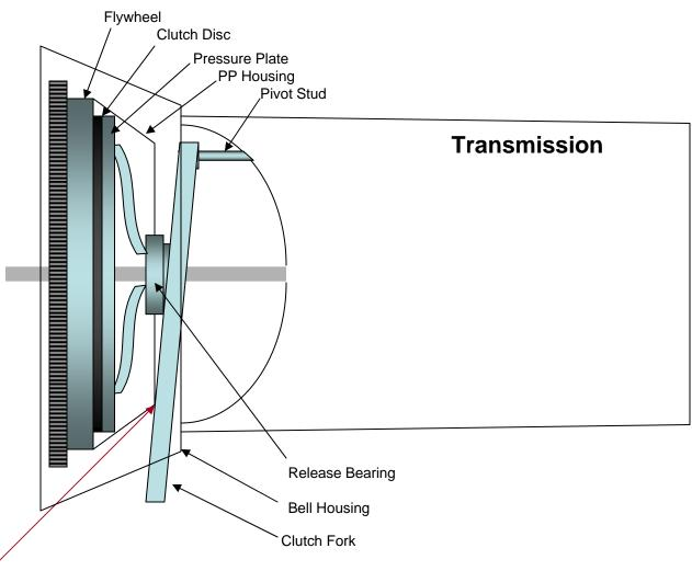
Interference w/ corner of PP housing HERE Prevents clutch disc from completely disengaging
