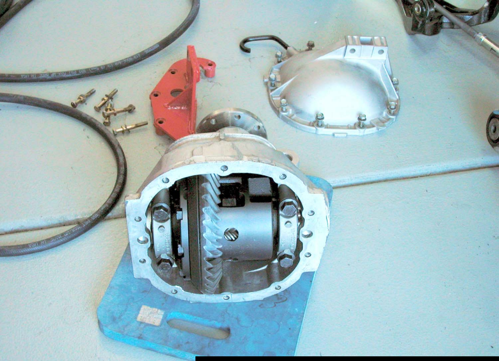
Torsen T2R & FRPP gears in diff housing
