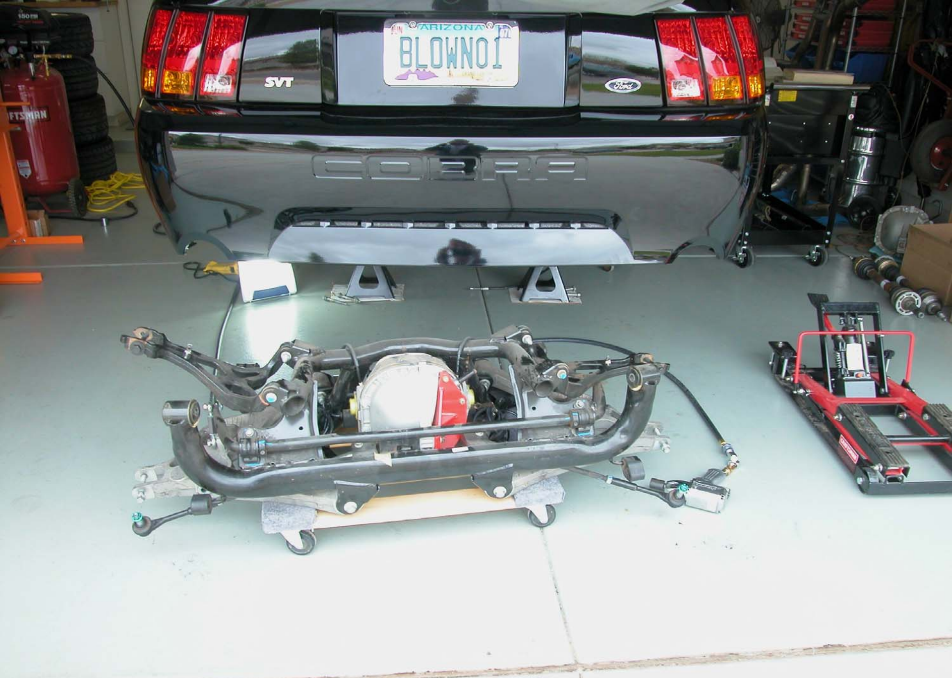
Stock '01 IRS w/ halfshafts removed
