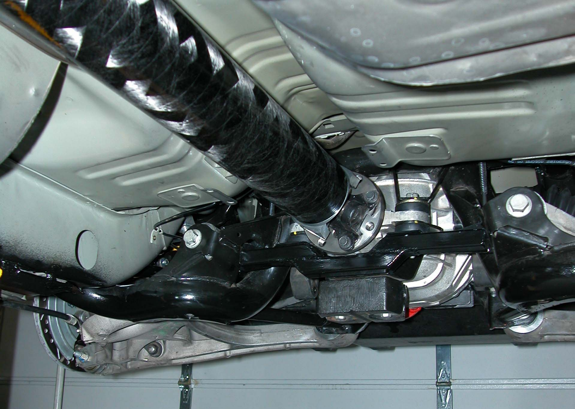
Driveshaft coupling bolted to pinion flange
