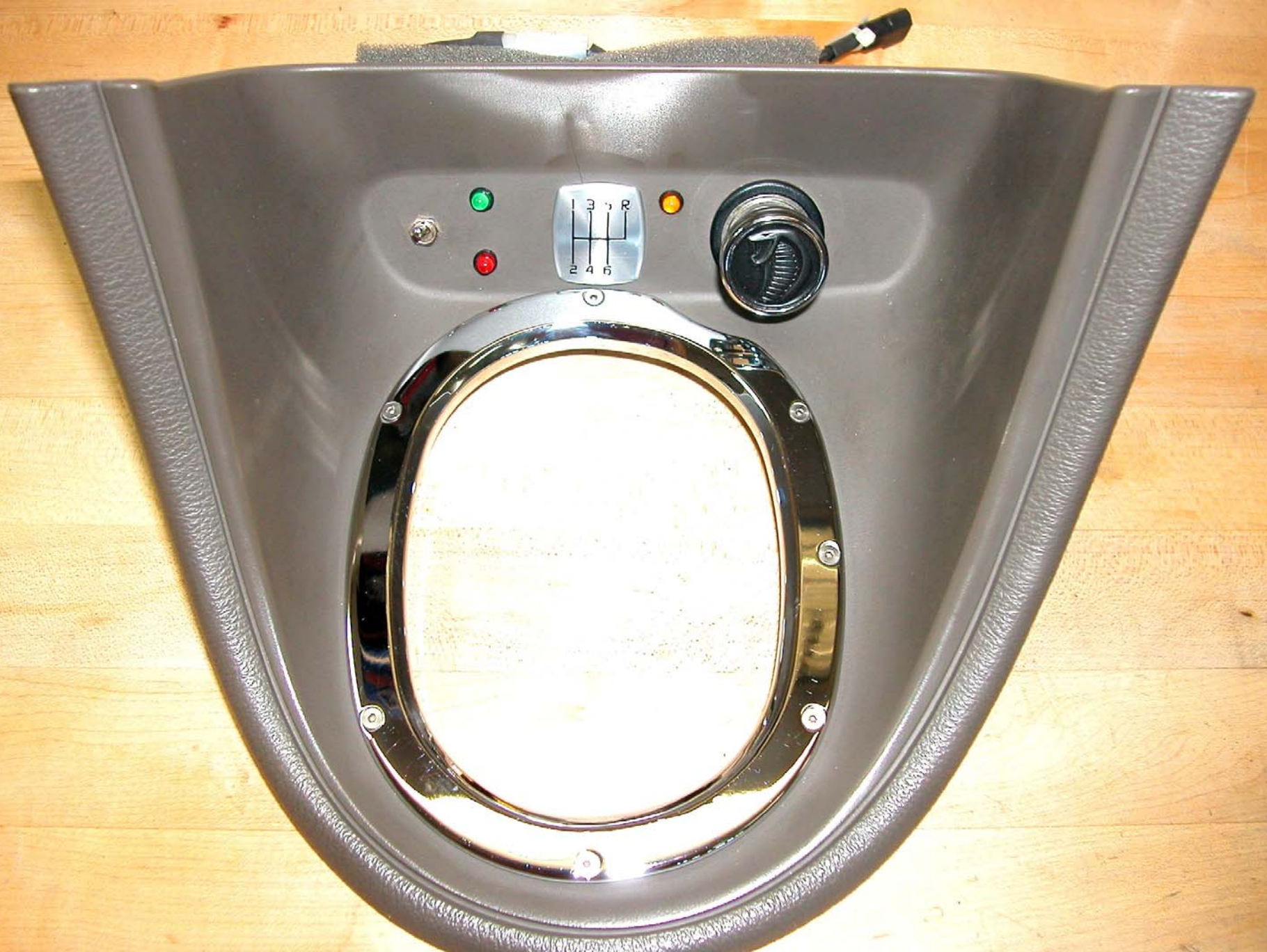
Console trim panel w/ T-56 shift placard & amber REVERSE LED added
