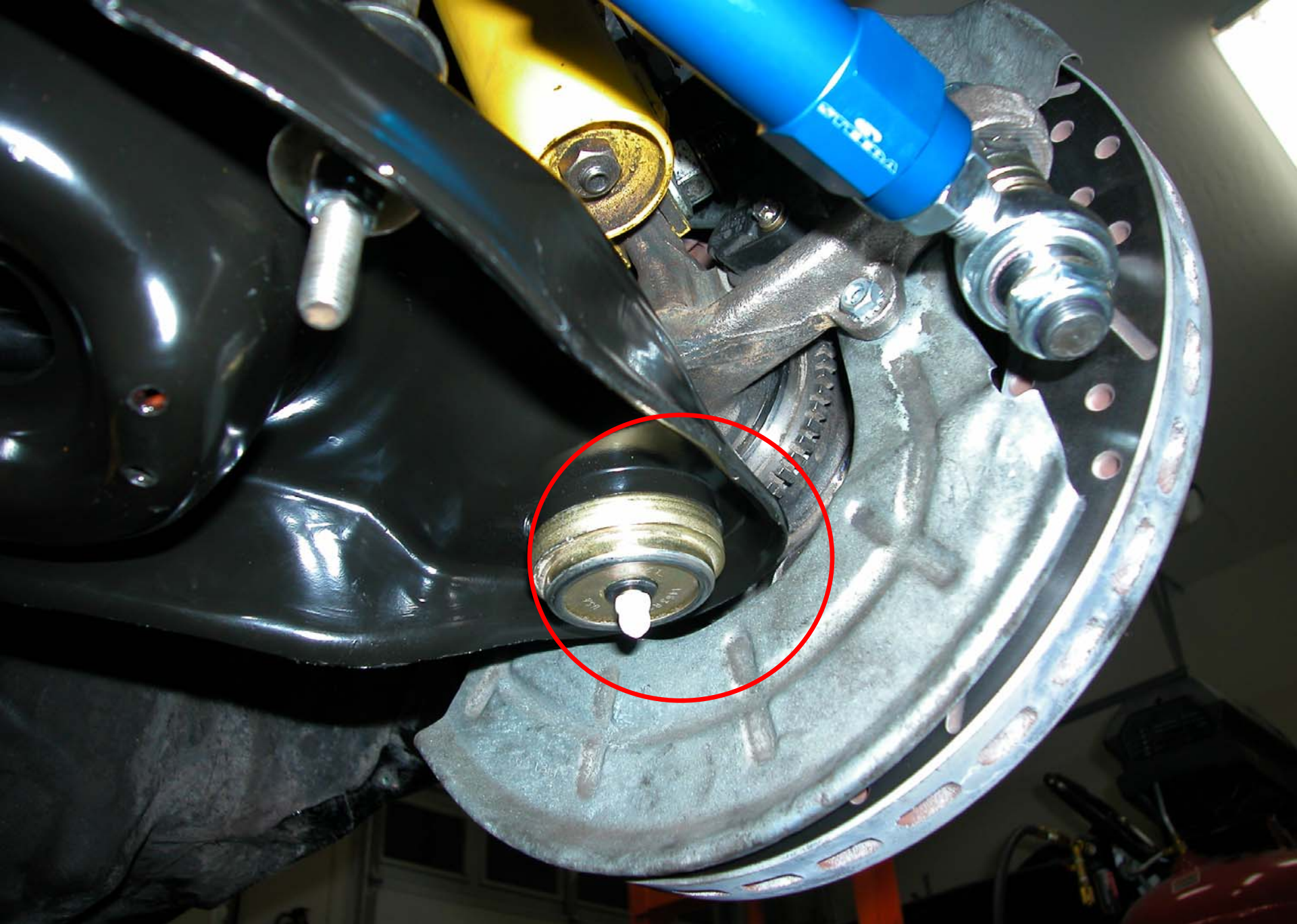
Third potential interference spot may require bending shield away from control arm
