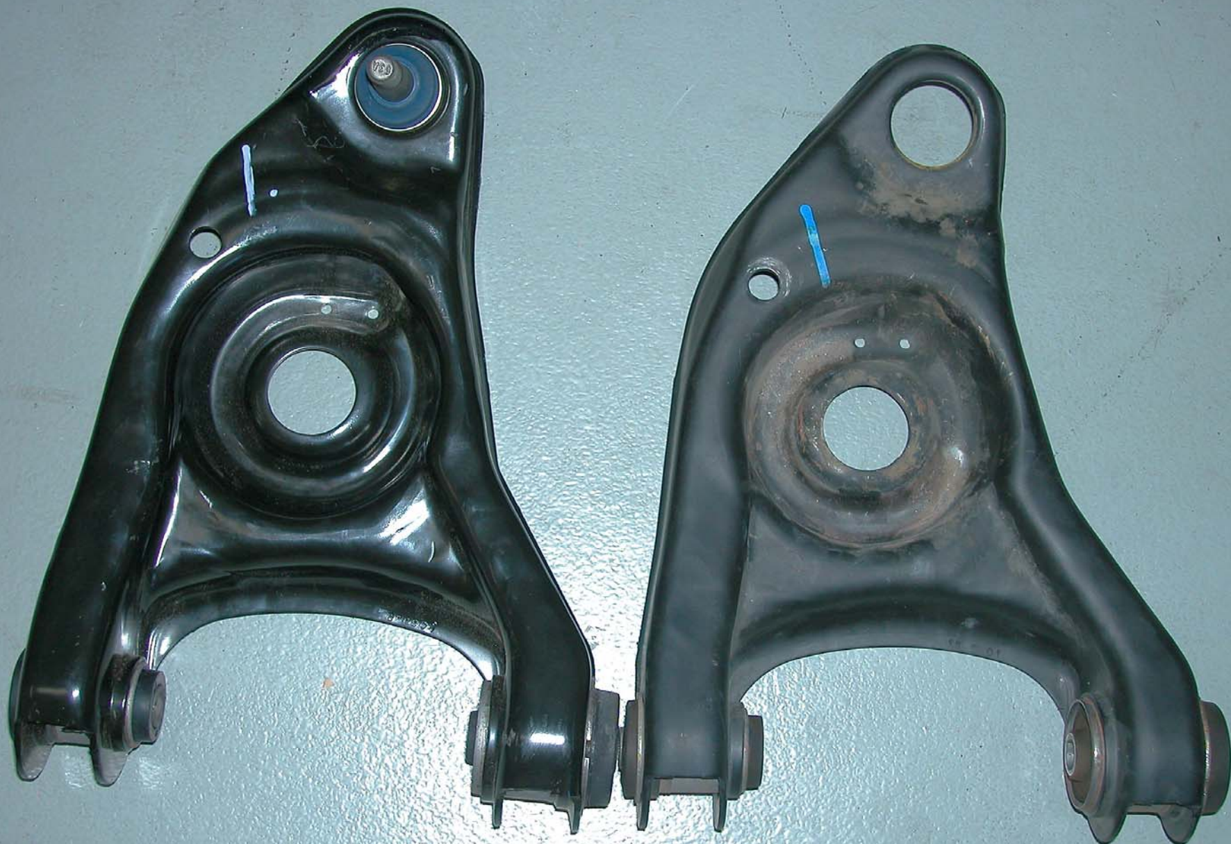
New front control arm w/ X2 balljoint next to original arm
