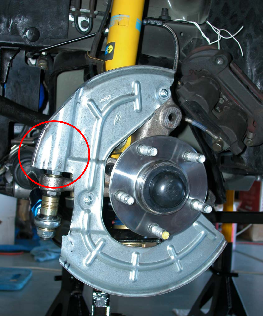
Left shield after cutting and mounting Red circle indicates a second potential interference point that can be eliminated by simply pulling the shield slightly away from the bolt
