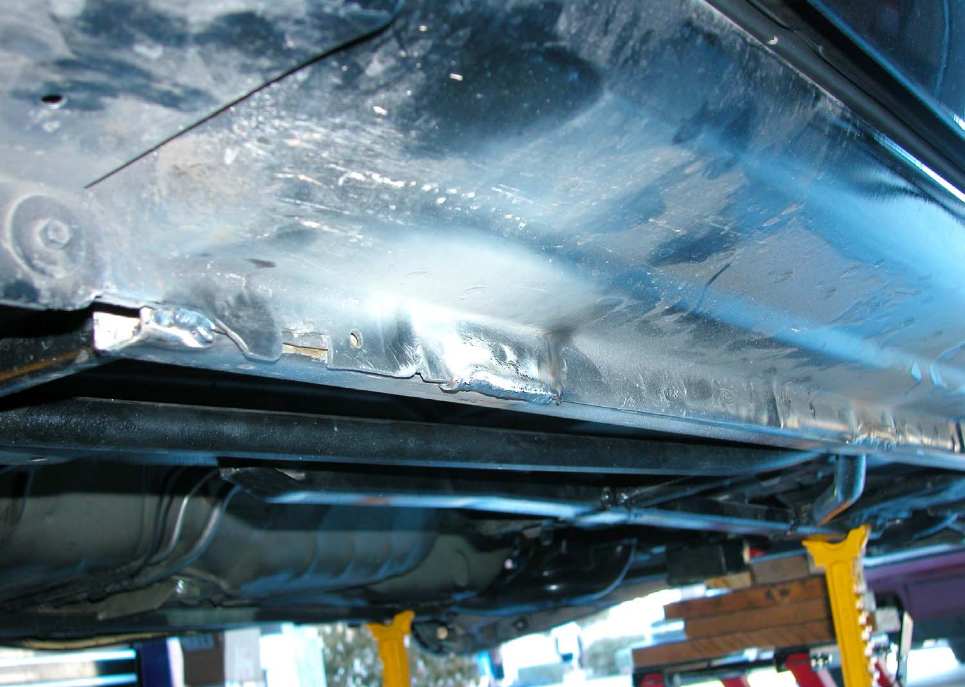
Proper welds along left jacking rail
