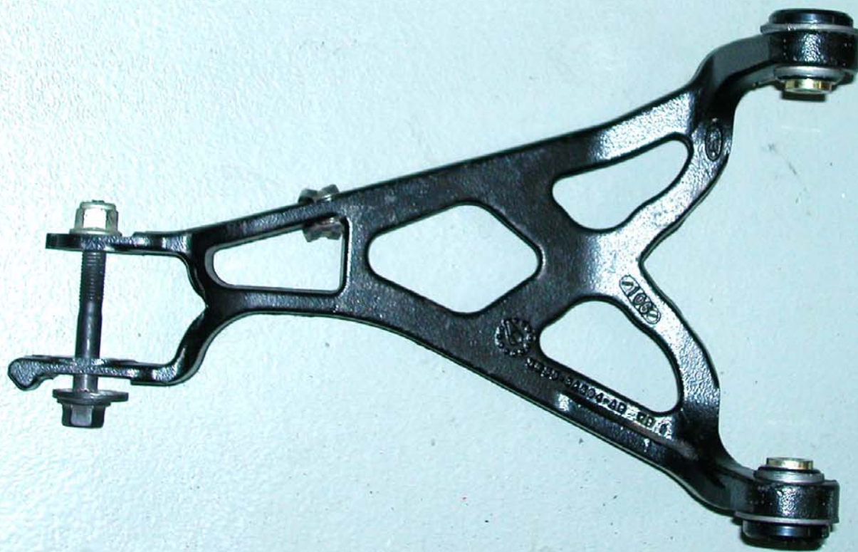
Rear tie rod w/ MM adjustable end & UCA w/ poly bushings
