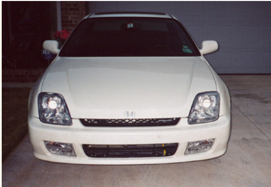
Johnny's 1998 Honda Accord with 6000K Audi TT projector retrofit:
