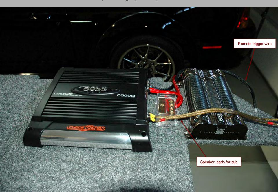
Amp wiring detail: NOTE: 4-gauge ground wire not yet connected
